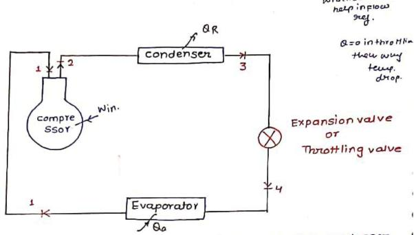
The basic components of v-c cycle are compressor, condenser, expansion valve, Evaporator.
