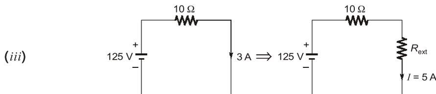
**Note:** Given data is incorrect, because by adding a resistor in series, the circuit current will decrease from 3 A.
