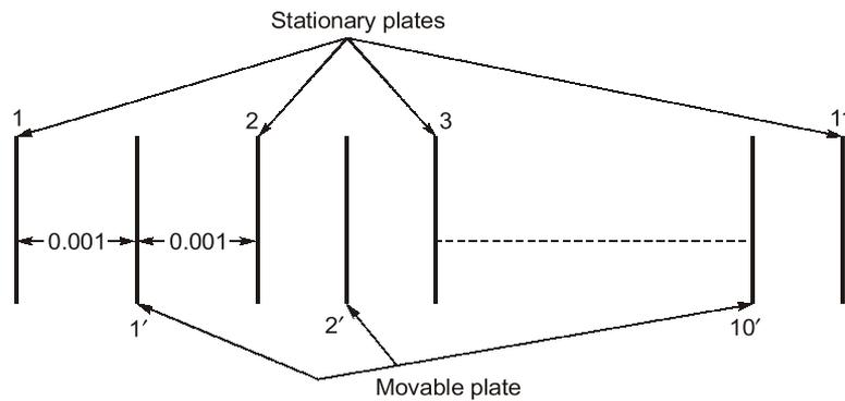
Total 20 capacitors will be formed using 10 movable and 11 stationary plates.
