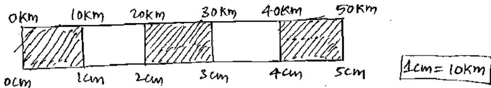
→ Graphical Scale is a line drawn on the plan (or) Map on which ground distance is directly marked.
