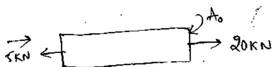
$$\sigma = \frac{\text{Resisting force}}{\text{Area}}$$
