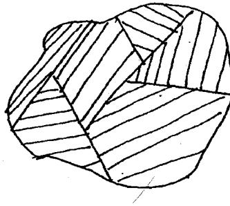
The atoms in the grains are arranged in an order but the grains are all differently arranged.
