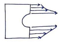
• For a plate with elliptical hole,  $K_t = 1 + \frac{2a}{b}$
