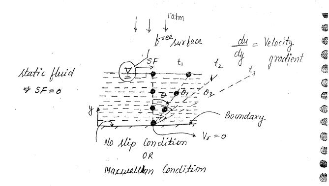
$\frac{d\theta}{dt} \rightarrow \text{Rate of angular deformation (Not Constant)}$   $S \rightarrow SOM$   $L \rightarrow \text{fluids (FM)}$
