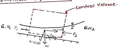
Net force acting an cv = P1-P2-Fs + wsin8 in the direction of flow.
