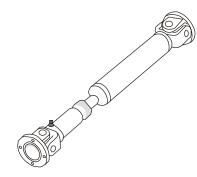
Propeller shaft is under compression due to thrust in X-Y.
