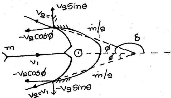
$\phi$ : Vane angle at exit
