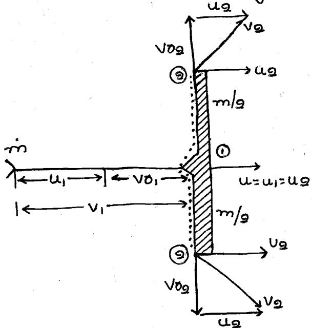
$v_{02} \ll v_1 \rightarrow$  Due to impulse force
