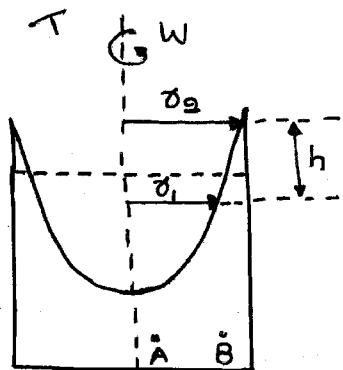
$$h = \frac{P_0 - P_1}{\rho g} = \frac{\omega^2 [v_0^2 - v_1^2]}{\rho g}$$
