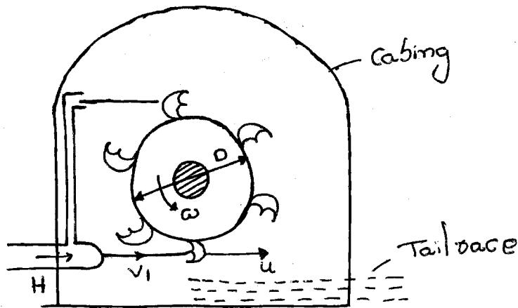
No hydraulic function  $\xi$  used to avoid the splashing of water
