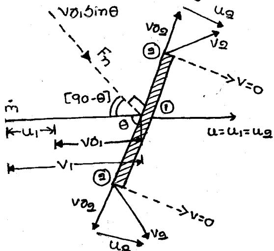
$$\dot{m} = \rho_a V_{01} = \rho_a [v_1 - u_1]$$
