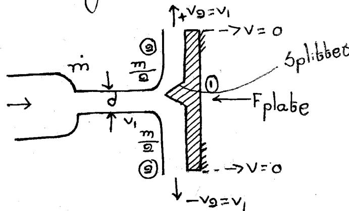
$$\frac{P_1}{\rho g} + \frac{v_1^2}{2g} + z_1 = \frac{P_2}{\rho g} + \frac{v_2^2}{2g} + z_2$$
