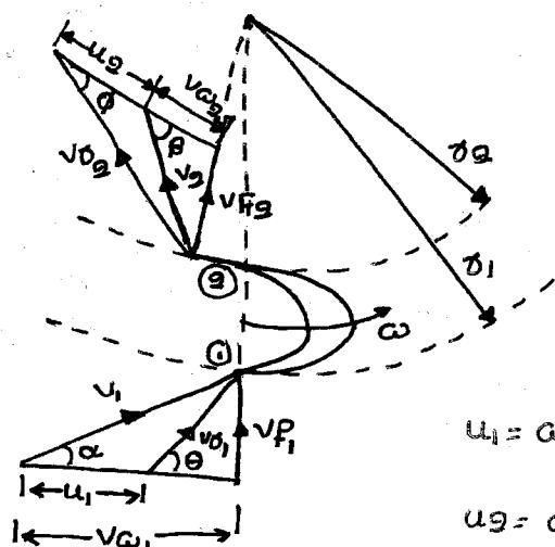
$$\begin{aligned}u_1 &= \omega r_1 = \frac{\pi d_1 N}{60} \\ u_2 &= \omega r_2 = \frac{\pi d_2 N}{60}\end{aligned}$$
