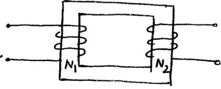
is @ stationary there is no rate of change of flux linkage. never work on DC.
