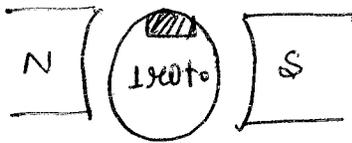
when conductors make one rotation then conductors will pass south pole and then also north pole. so, if south pole produce one pulse then north pole produce opposite. [There is no rule is south pole producing + or -ve & north pole producing +ve or -ve]
