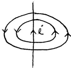
current carrying conductor producing concentric flux line [Right hand Thumb rule] By using R-H thumb rule fingers represent flux line direction and thumb in the current direction.
