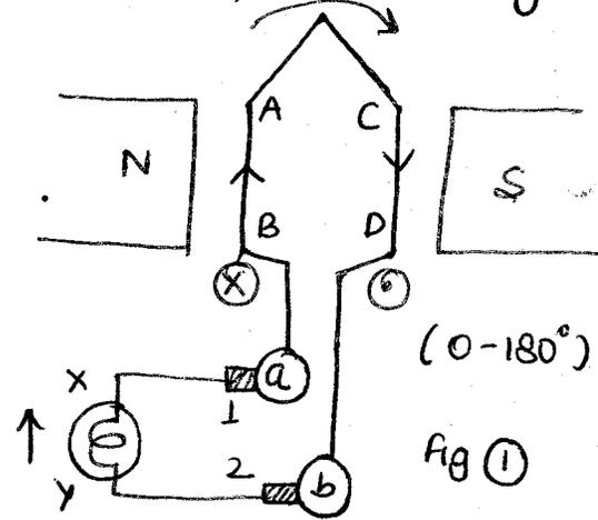
current direction  $\rightarrow$   $\underline{BACD}$   $\underline{b2y1aB}$
