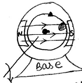
Place a conductor on rotating part & don't rotate the rotating part then there is flux and conductor but missing the rate of change of flux linkage
