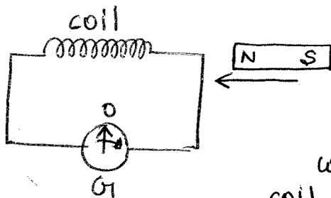
When the magnet is stationary then [near the coil] galvanometer is deflecting zero.
