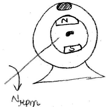
Rate of change of flux linkage occurs in conductor which produces dynamically induced emf.
